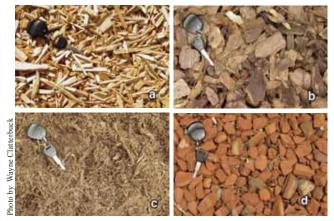
Different types of mulches: (a) wood chips, (b) pine bark nuggets, (c) shredded hardwood bark and (d) brick chips.
